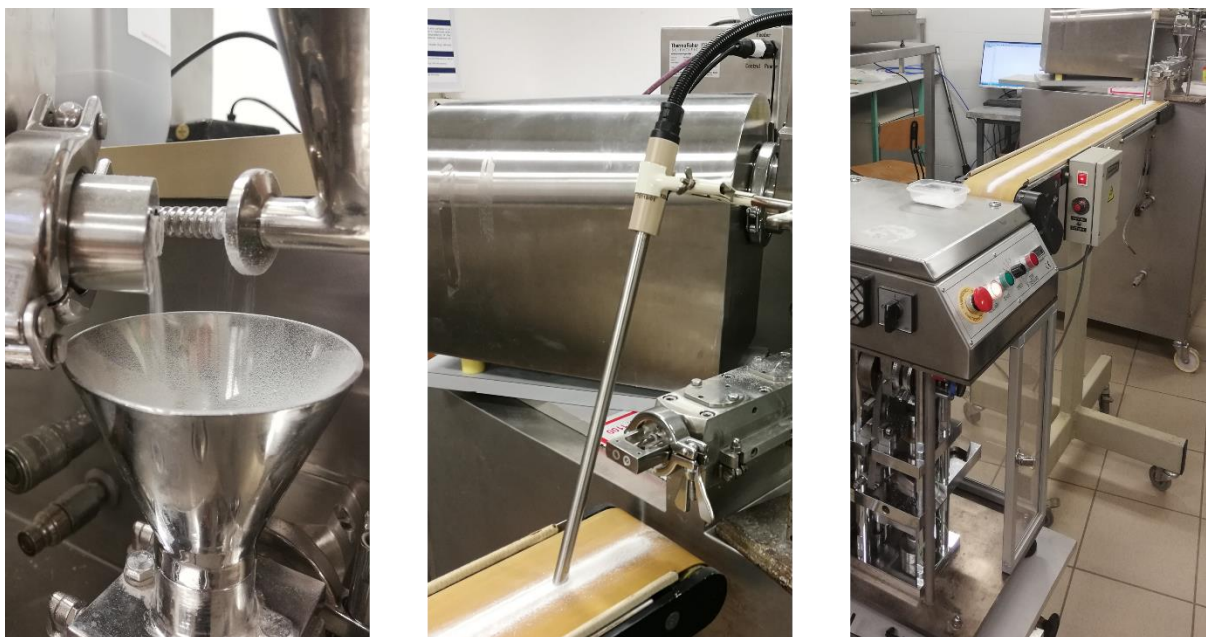
Figure 40. Feeding of MCC and ASA into the hopper of the continuous blender (left); NIR probe mounted above the belt conveyor after blending (middle); continuous blender, belt conveyor and tableting machine integrated in one CM line (right).
