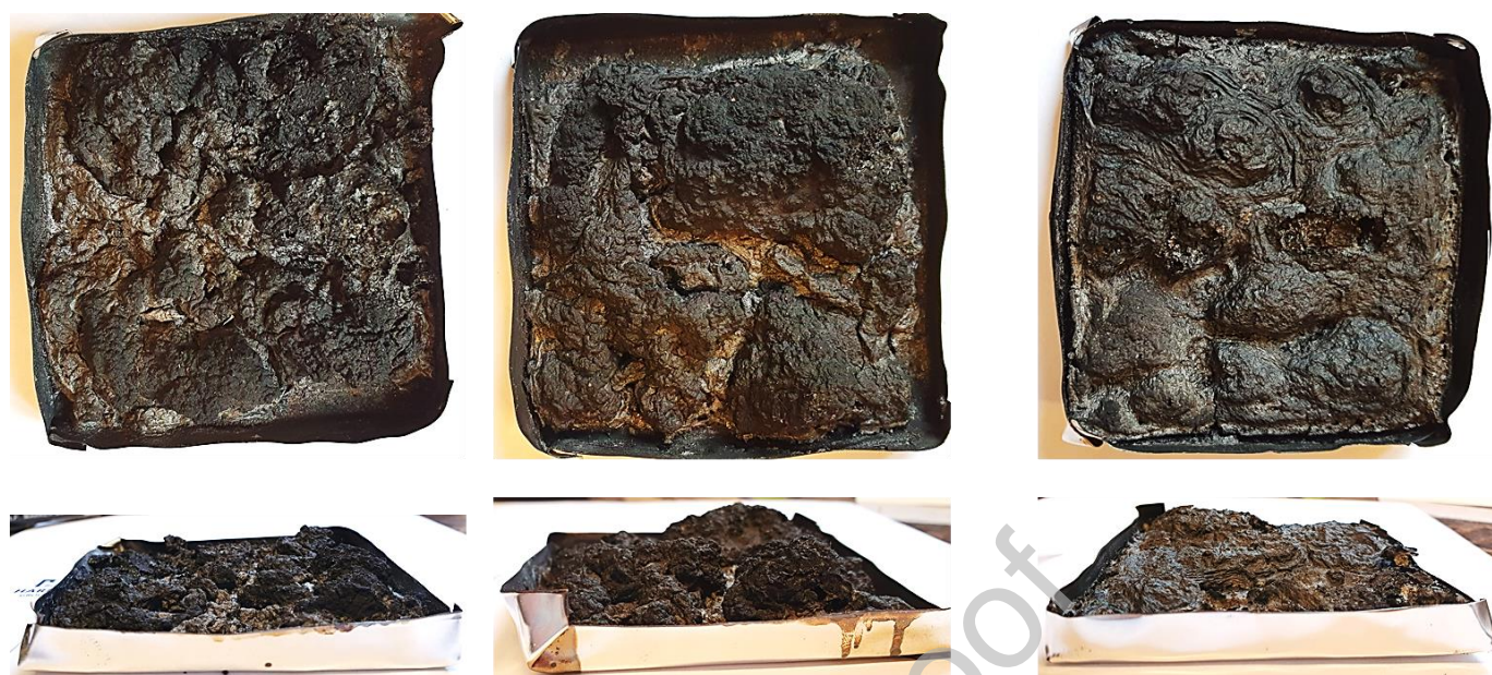
Figure 10 The charred residues obtained after cone calorimeter tests from left to right: PLA/APP; PLA/APP/HP- \beta -CD powder; PLA/APP/HP- \beta -CD fibre
