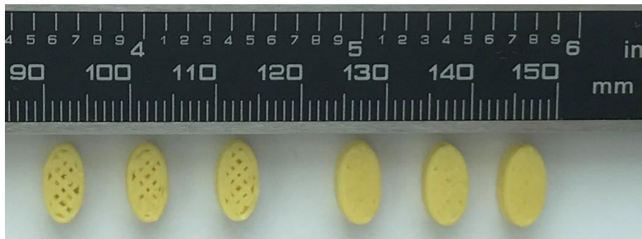
Fig.4.1. Photographs of 10% lumefantrine 3D-printed tablets (H0: 10% lumefantrine - 90% HPC SSL) with (left) 80% and (right) 100% infill density
