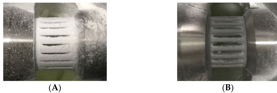
Figure 3. Product particle adhesion of theophylline at the classifier wheel after micronization: (A) without additives and (B) with 1 wt.% SSF.
