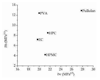
Figure 7. Bagley diagram [32] for the five polymers used for the preparation of tandem films.
