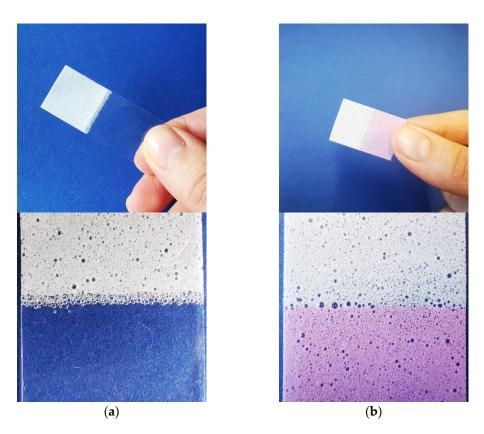
**Figure 9.** Applicator films with a (**a**) water-insoluble EC applicator and (**b**) water-soluble PVA applicator. The pictures were taken in front of a blue background.
