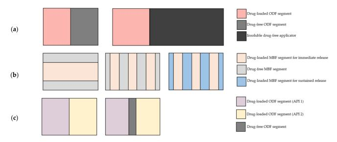
**Figure 1.** Conceptualization of different tandem films and their possible applications: (**a**) applicator films, (**b**) optimization of dissolution rate and (**c**) optimization of stability in the case of incompatible APIs.
