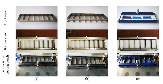
**Figure 2.** Comparison of the insert types in the front and bottom views and installed on the coating bench: (**a**) precursor steel model, (**b**) optimized steel model and (**c**) 3D-printed model.
