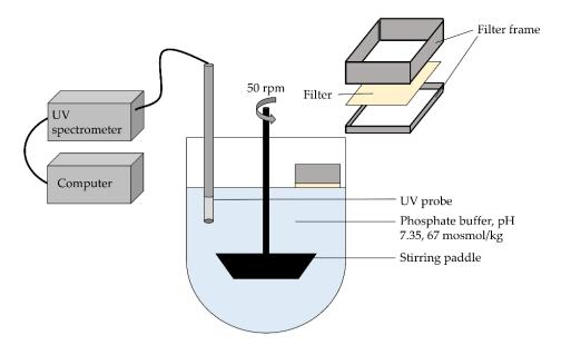
**Figure 3.** Setup for dissolution testing of the oral films, modified from Krampe et al. [43] with kind permission from Elsevier.
