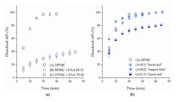
**Figure 11.** Dissolution profiles of (**a**) mucoadhesive conventional and (**b**) tandem films in comparison to the HPMC "reference" film (n = 3, mean  $\pm$  sd).
