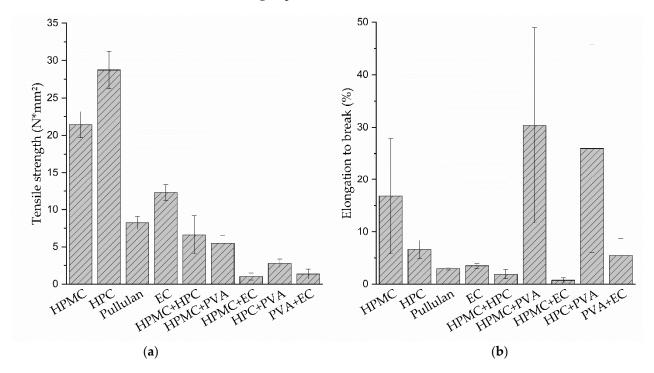
**Figure 5.** (a) Tensile strength and (b) elongation to break of the original formulations and the successfully prepared tandem films (n = 6, mean  $\pm$  sd). The PVA films did not rip until reaching the tensile tester's maximum distance (elongation > 300%).
