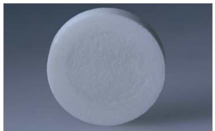
Pic. 2. Tablet Defect on Tablet Lubricated with Magnesium Stearate
