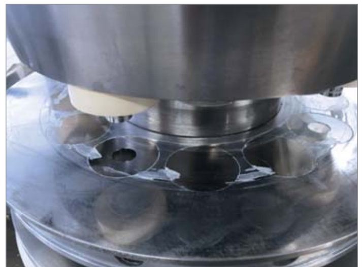
Pic. 1. Sticking of Powder Mixture with Ibuprofen and Sodium Stearate
