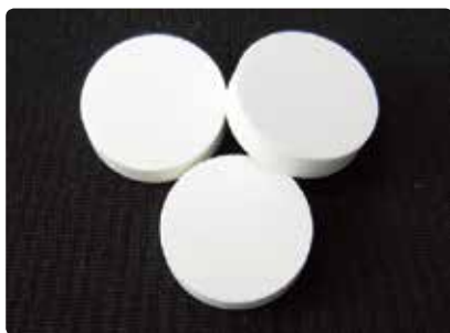
Linseed oil tablet, Ø11.3mm, 125N at 500 kg/cm 2
