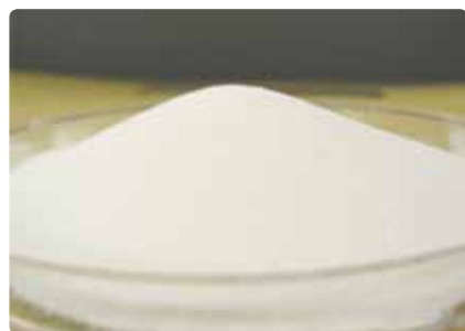
Neusilin® US2 +30% linseed oil, Dry at 50°C
