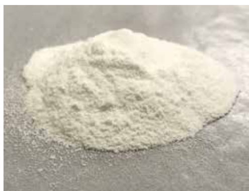
FujiSil™-F powder loaded with Vitamin E oil (FujiSil™-F:Oil = 1:1)
