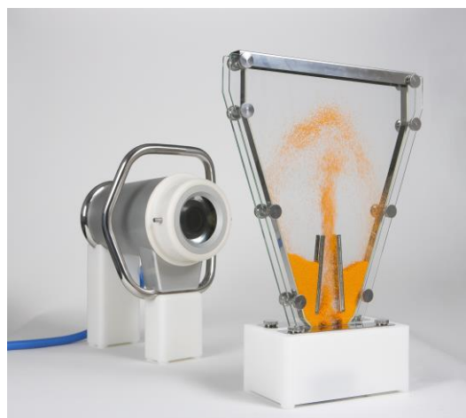
Figure 1: Image acquisition of pellets in a 2D fluid-bed system (right) with visual inspection system PATVIS APA (left).
