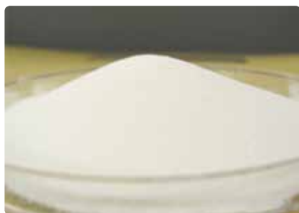
Neusilin® US2 +30% linseed oil, Dry at 50°C
