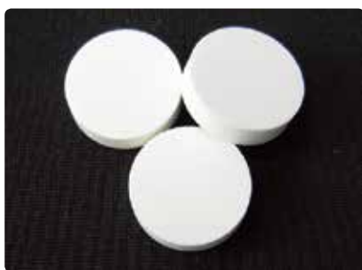
Linseed oil tablet, Ø11.3mm, 125N at 500 kg/cm 2
